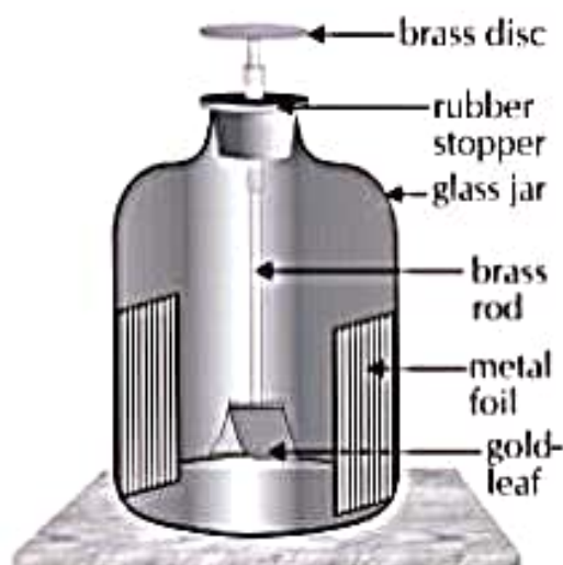
Fig. (a) Gold-leaf electroscope
